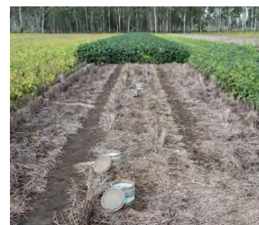
Nitrous oxide chambers in the cropping trial. Source: Prof. Phil Brown CQUniversity, 2014
