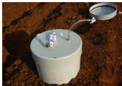
N 2 O Chamber with sampling apparatus. Source: Z.Nicholls, 2014
