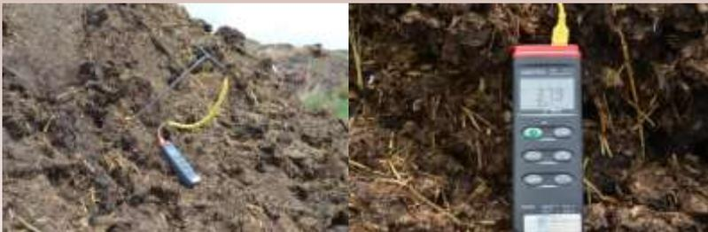
Figure 3 - Long stemmed thermometer to measure windrow temperature and composting activity.
