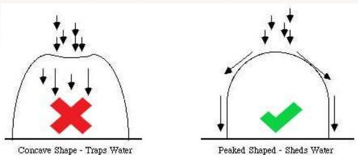
Figure 1 – The peaked shape on the right is ideal as it is built to shed water.
