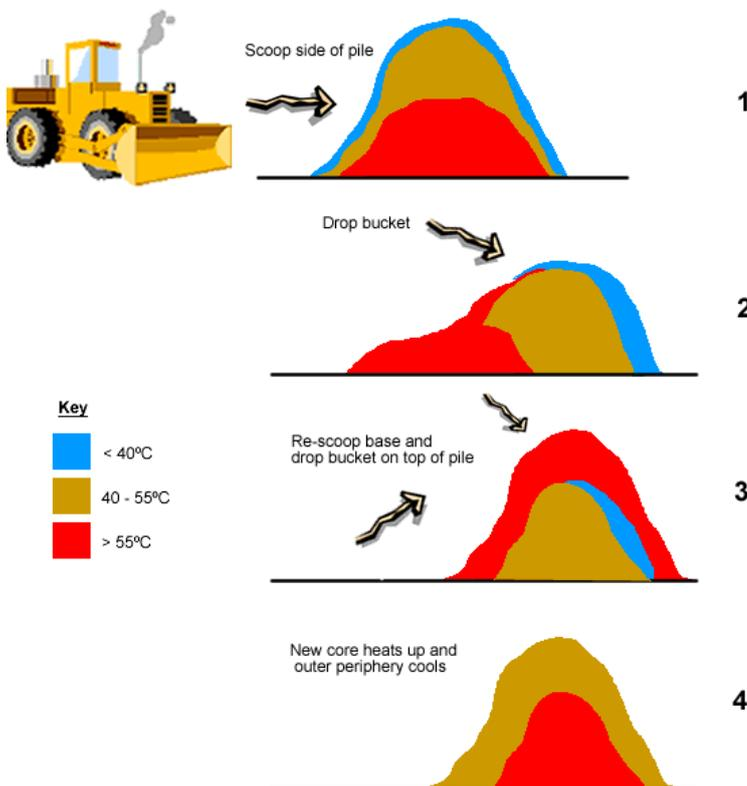
Figure 4 - Mixing the various zones of the windrow after pasteurisation temperature has been reached.
